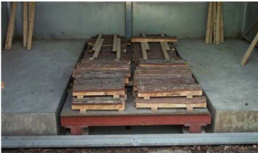
Figure 4 . The Thetford material being loaded in to the kiln for drying to 12% moisture content
